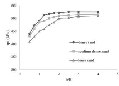
Fig 5. Effects of geogrid layers width on bearing capacity of in sandy soil in several density.
