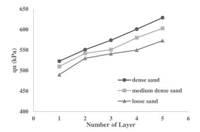
Fig 10. Effects of number of geogrid layers on bearing capacity in sandy soil at several density.
