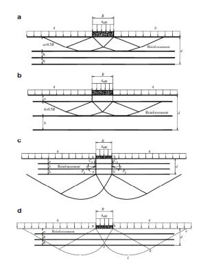
Fig 1. Failure modes of reinforced soil foundation, (a) Failure above top layer reinforcement [9], (b) Failure between reinforcement layers [10], (c) Failure similar to footings on a two-layer soil system [10], (d) Failure within reinforced zone.
