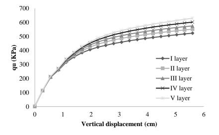
Fig 9. Effects of number of geogrid layers on bearing capacity of in dense sand.
