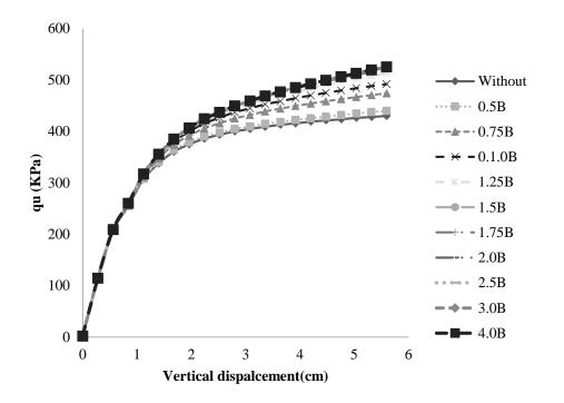
Fig 4. Changes of ultimate bearing capacity of foundation versus vertical displacement for values of geogrid layers width in dense sand.
